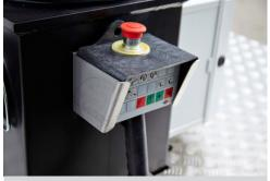
Lower control panel (wired remote control panel)
