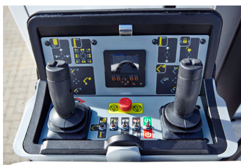
FPC (Full Proportional CANbus controls): Variable outreach (with load cell) and up to 4 actions at a time
