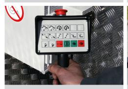
Lower control panel (wired remote control panel)
