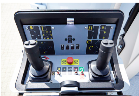
LMC (Load Moment Controls): Variable outreach and up to 2 actions at a time (1 per joystick)
