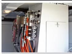
Ground level emergency lowering from the load area (pedestal mounted valve bank)
