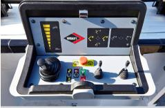
RLC (Relay Lefthand proportional Controls): Fixed outreach and 1 action at a time
