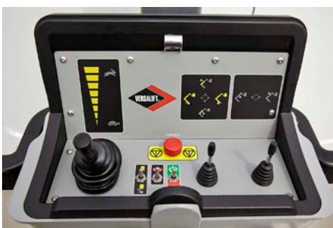
RLC (Relay Lefthand proportional Controls): Fixed outreach and 1 action at a time
