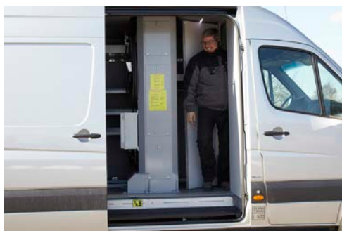
Walk-Through-System: Direct access from the cabin to the bucket through the vehicle (optional)
