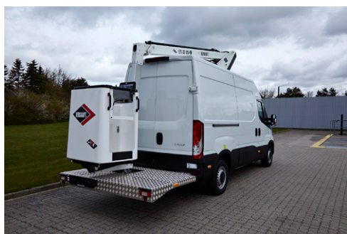
Rear platform (Bucket stowed asymmetrically)
