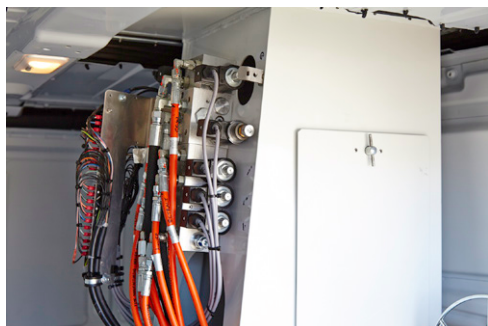
Ground level emergency lowering from the load area (pedestal mounted valve bank)
