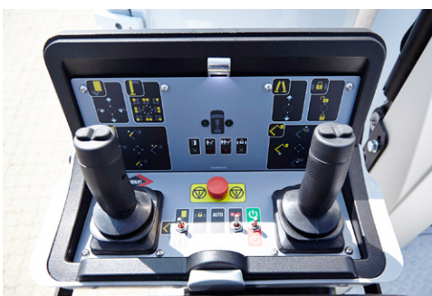
LMC (Load Moment Controls): Variable outreach and up to 2 actions at a time (1 per joystick)
