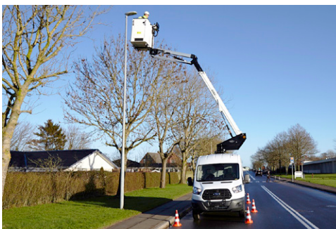
Turret/knuckle tail swing and outriggers within the mirrors
