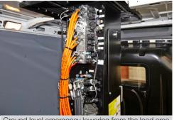
Ground level emergency lowering from the load area (pedestal mounted valve bank)
