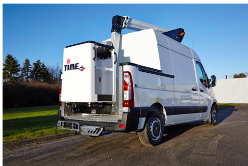
The bucket is stowed in the cutaway section of the van for compact transport dimensions
